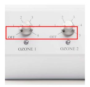
**Step 5.** Turn off Ozone Generator and oxygen source.
