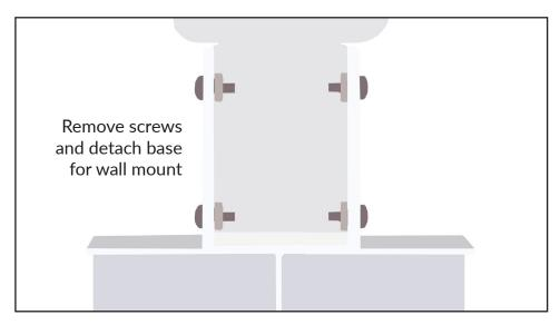
Due to the variation across buildings, mounting hardware is not included. Using the mounting holes in the back of the stand, screw directly into a wall stud or use heavy duty wall anchors. A level is recommended to make sure the stand is properly mounted.
