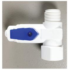
**Note about the blue handle:** The handle on the valve makes it easy to temporarily stop water flow to your filter system in order to change filters or perform other maintenance. If the valve is pointed up, water flow is shut off to the filters. If it is horizontal, water can flow into the filters.
