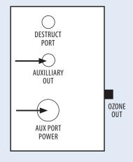
the Ozone Out port, then use the Aux port to fill a syringe without unhooking your bubbler.
