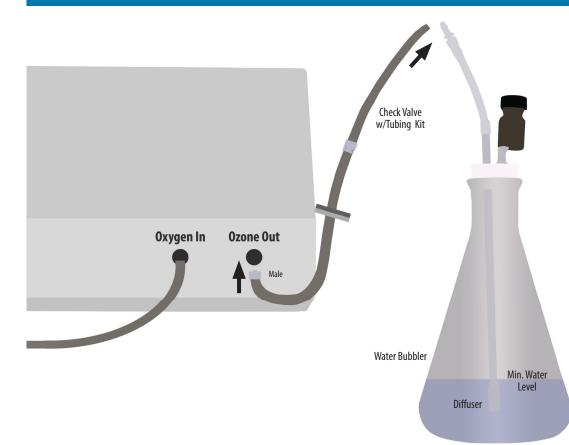
1. Fill the bubbler with at least as much water as is needed to cover the white diffuser (see diagram).
