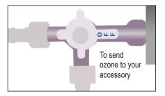
You can also attach the ozone cup **directly to the Ozone Out port** on your ozone generator using the check valve and tubing kit. If you do this, we recommend lightly wetting the area to be treated before using the cup.
