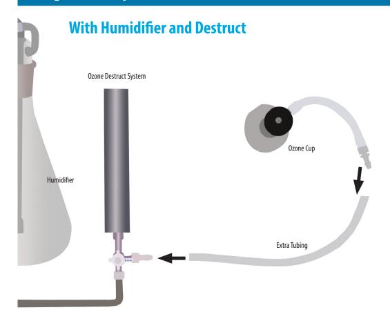
1. Attach an extra piece of tubing to the ozone cup and attach the other end to the ozone destruct as shown. Make sure the dial is turned toward the cup until you're ready to use it.
