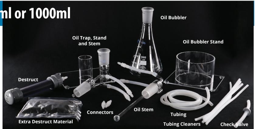
**What you need for a standard setup:** Destruct, Check Valve, Tubing, two Luer fits, Oil Trap and Oil Bubbler. Extra Destruct Material and Tube Cleaners can be put aside until you need them.
