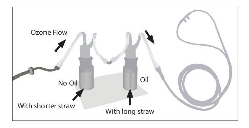
Connect the nasal cannula to the oil bubbler.
