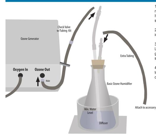
1. Fill the bubbler with at least as much water as is needed to cover the white diffuser (see diagram). If your humidifer came with a stand, place it in the stand.
